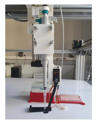
Figure 5: A real-life photograph of the developed end effector system integrated into the Cartesian robotic platform
