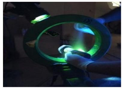
Figure 2: Magnetizing the material
